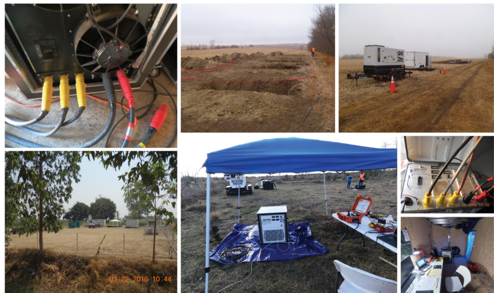
Figure 9. Field images of various components of the transmitter equipment. At the top left is the power connection of the 150 kVA transmitter switch box (back view). Its front view in the field is shown in bottom center. At the top center are pictures of the electrode pits where the current injecting electrode are buried. At the top right is a view of the 150 kVA generator and observer trailer (switch box is inside) used for 24 h continuous for 5 weeks operation partially at minus 20 °C. An inside view of the trailer is at the bottom right. On the left side is a transmitter site set up as camp in the tropic in an oil field.
